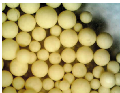
Fig. 2. Experimental modified sample of solid-phase extractant based on TODGA.
