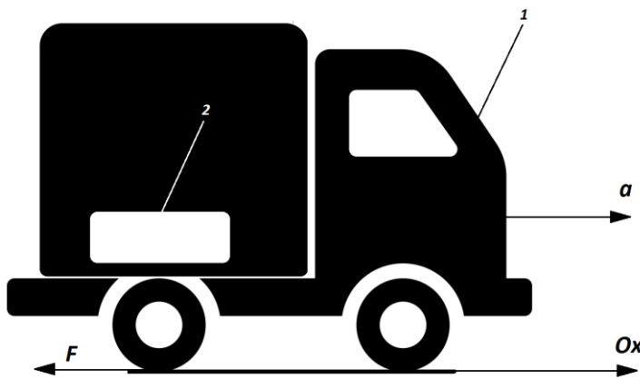
Figure 2. Scheme for the implementation of the dynamic method for controlling of weight of cargo transported by vehicle: 1 – vehicle; 2 – cargo.
