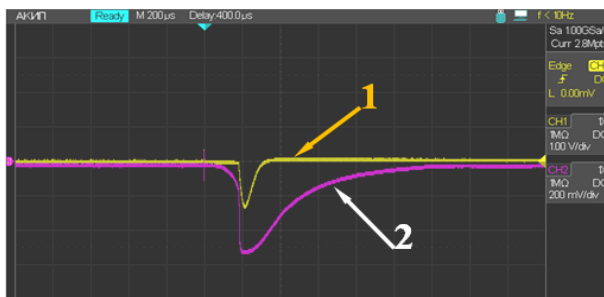
Figure 1. Dynamics of changes in current (1) and intensity of thermal radiation (2) of the processed material.
