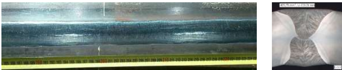
Figure 1 – Outer appearance and cross-section of a SAW-weld. Outer layer welded with the following wire configuration: d_{1,2} = 4.8 mm und d_{3,4,5} = 4 mm
