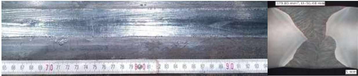
Figure 2 – Outer appearance and cross-section of a SAW-weld. Outer layer welded with the following wire configuration: d_1 = 3.2 mm und d_{2,3,4,5} = 4 mm
