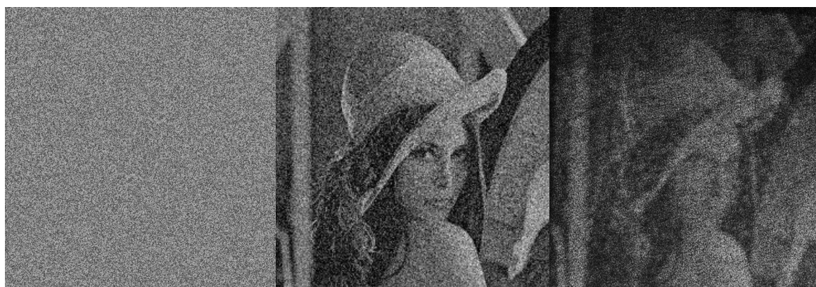
(a) Binarized hologram (b) Computer reconstructed image (c) Optically reconstructed image
