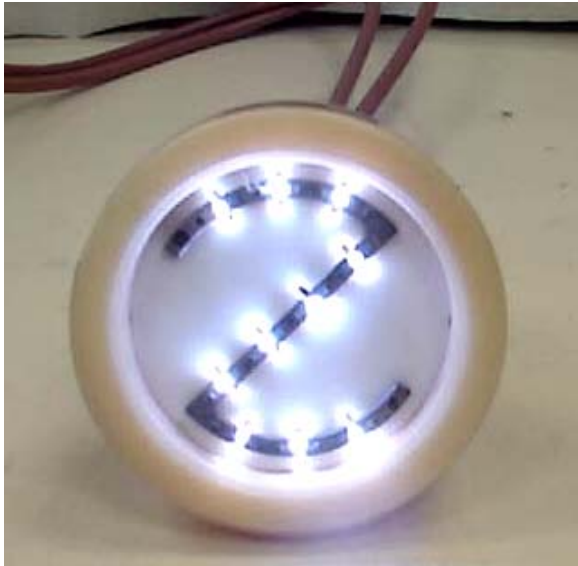
Fig. 5. Photograph of integral lighting for one pulse of a multigap electric discharge on the obverse side of the applicator.
