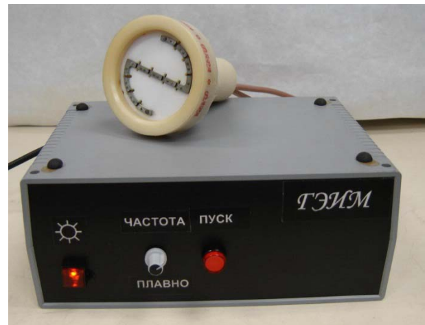
Fig. 3. General view of “Game” device, the supply unit and applicator on it.
