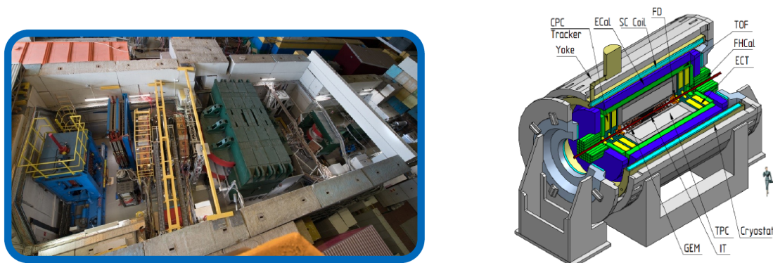
Figure 2. Left: View of the BM@N detector setup in a first experimental run in 2017. Right: Schematic layout of the Multi-Purpose Detector (MPD) for the first stage of the experiment expected in 2022.
